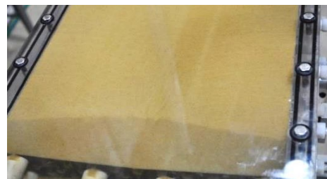
Figure 9. Arc-shaped slope formed by v-notch.
